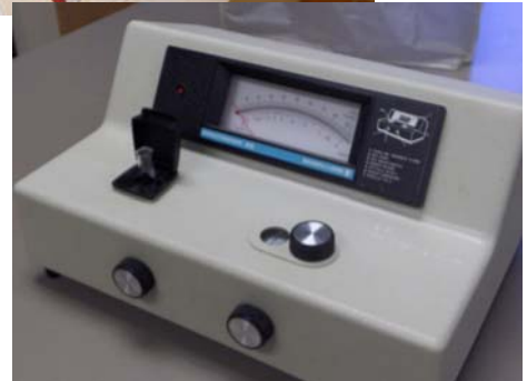
A spectrometer used for water quality testing
